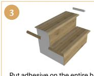
Put adhesive on the entire back of the stair tread and and fixed to the steps.
